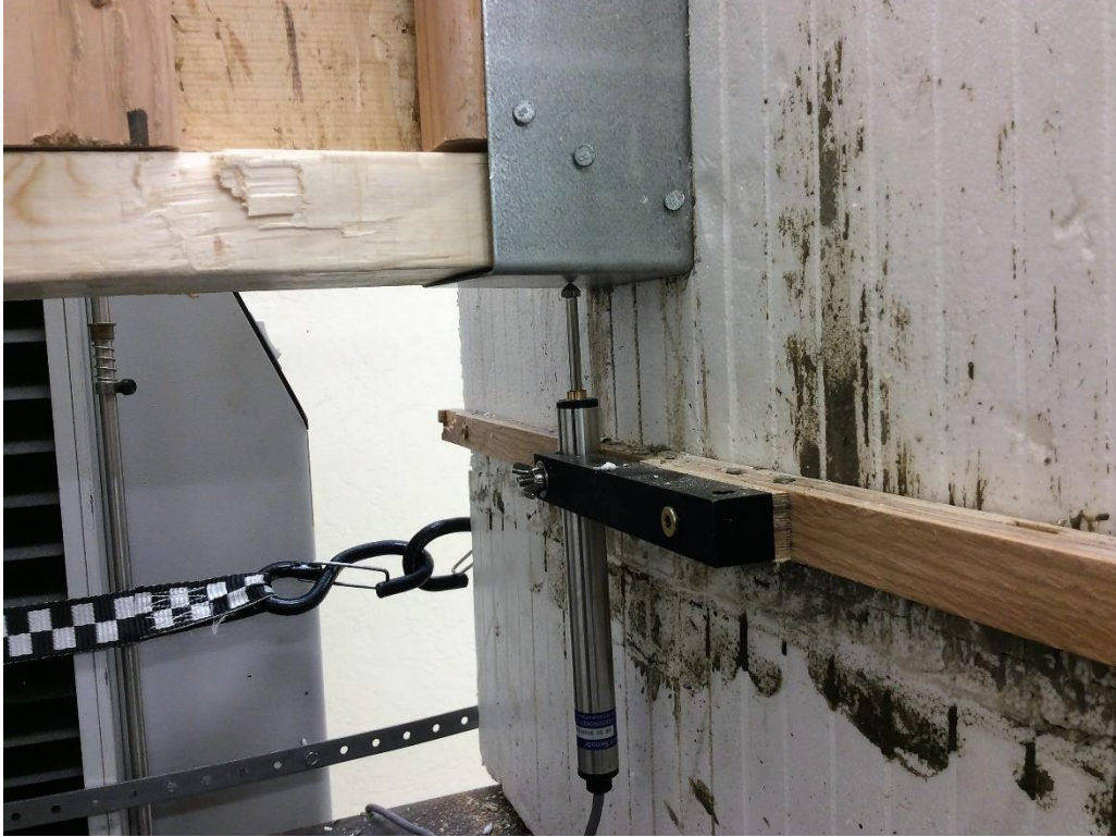
Figure 3. Test Setup- Right Joist Hanger
