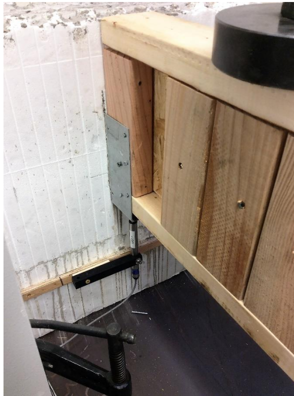
Figure 4. Test Setup- Left Joist Hanger
